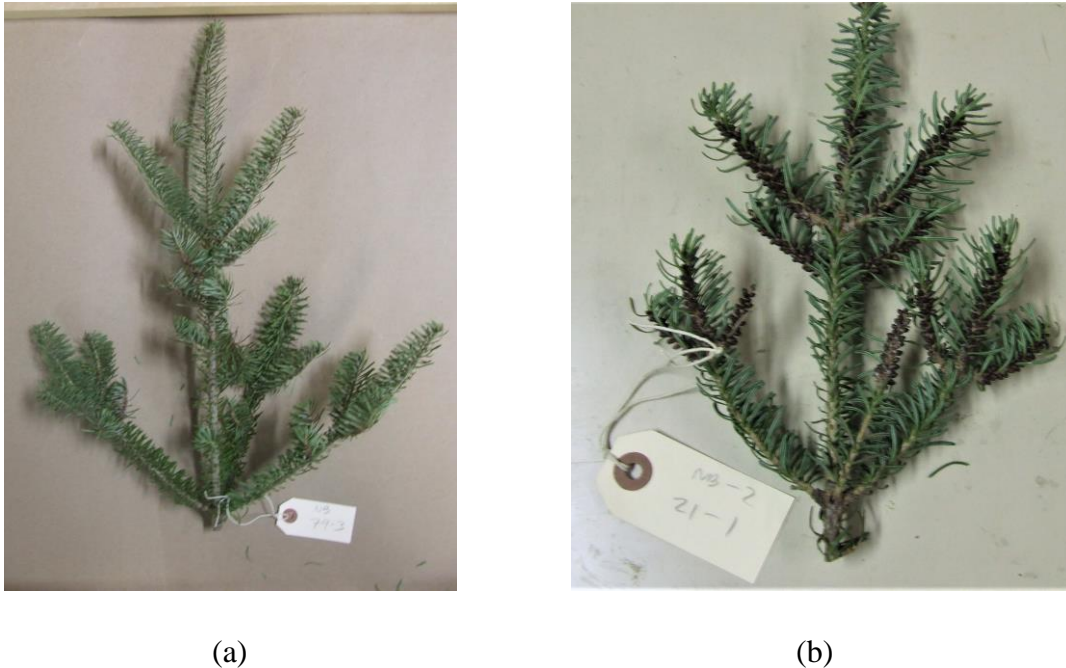
Figure 2. Needle retention branches cut to length. Branches with a low amount of pollen buds (a) and with a high amount of pollen buds (b).
